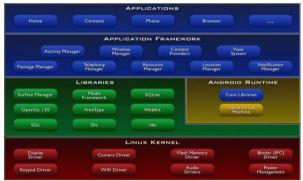
Fig 1. Android System Architecture [11]
